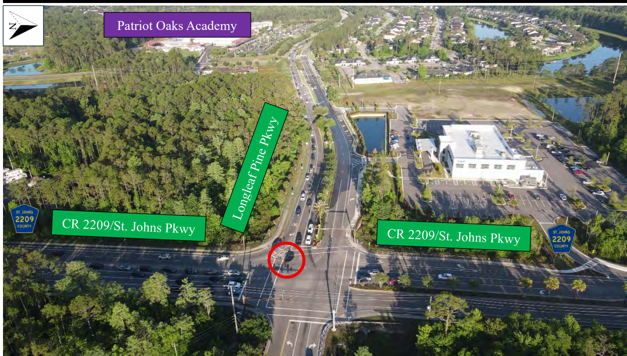
Vehicle using the eastbound through lane to turn right at St. Johns Parkway (CR 2209) in the AM peak hour
