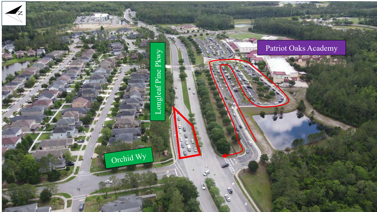
Light westbound queues observed in the PM peak period during school pickup time with crossing guard controlling the intersection
