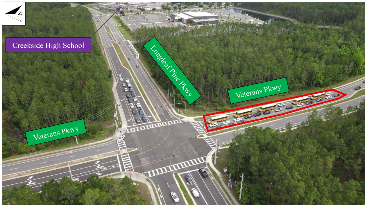
Northbound through queues with school buses were observed during PM school peak hour
