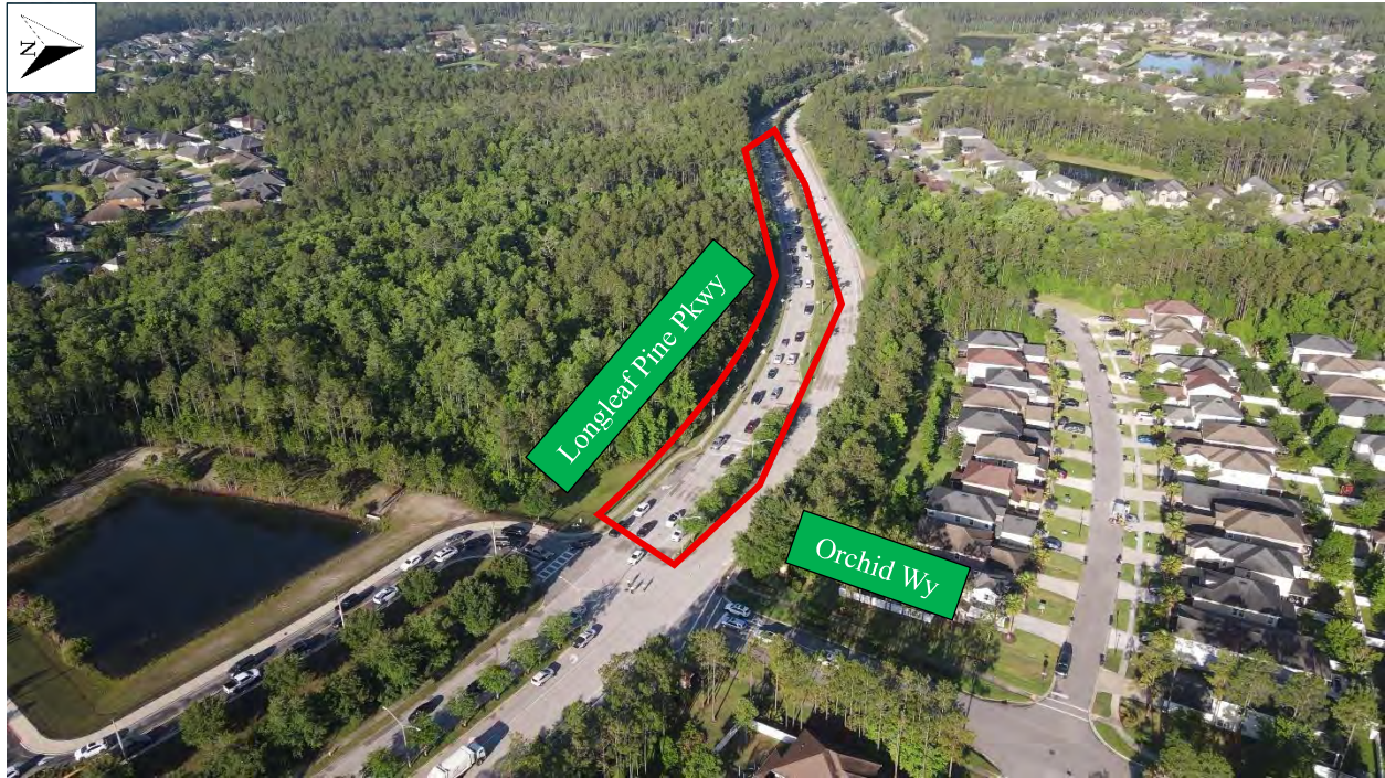
Long eastbound queues observed in the AM peak period with crossing guard controlling the intersection during school drop-off time
