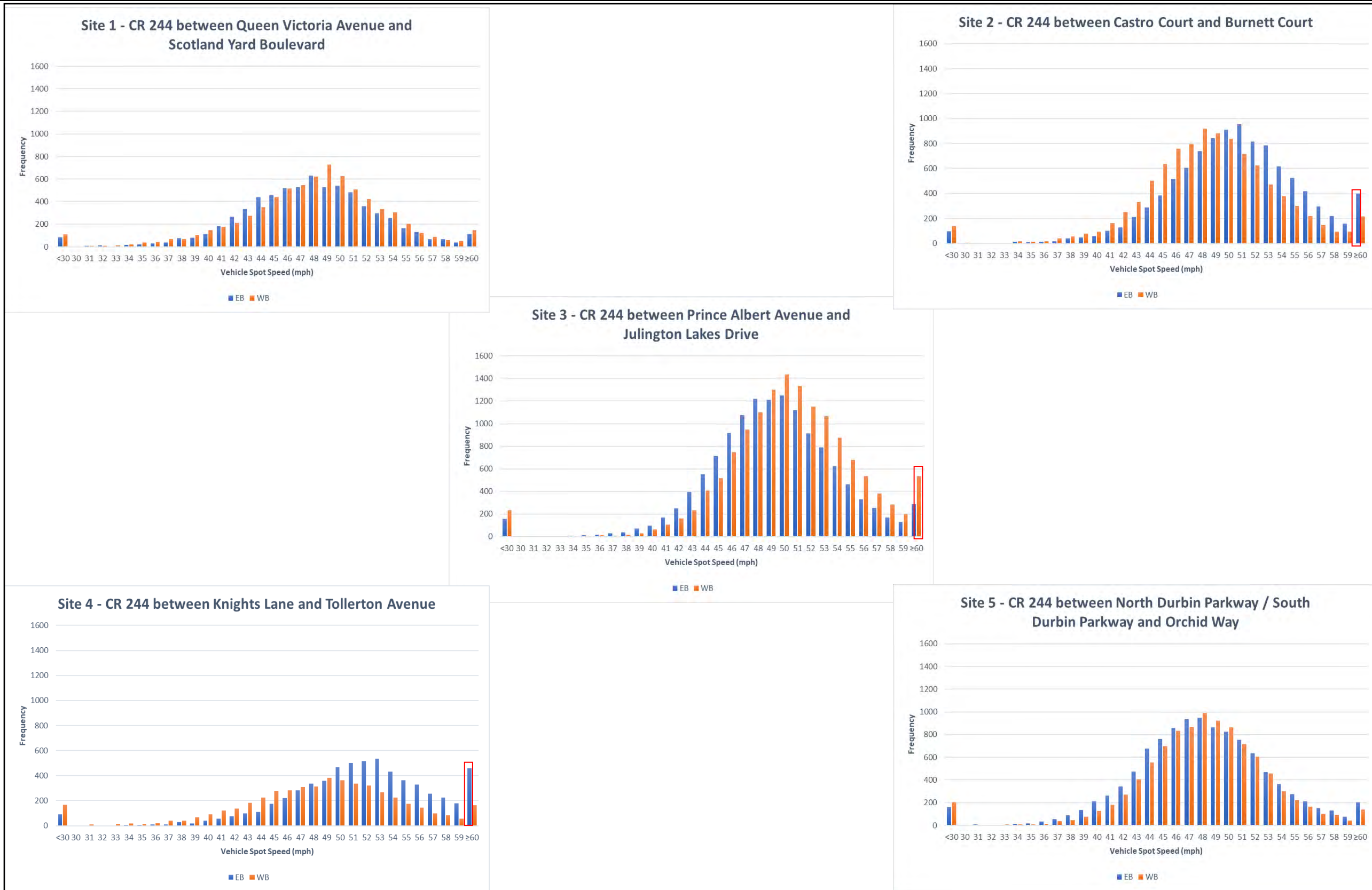
Figure 7: Spot Speed Histograms – Speed Frequencies
